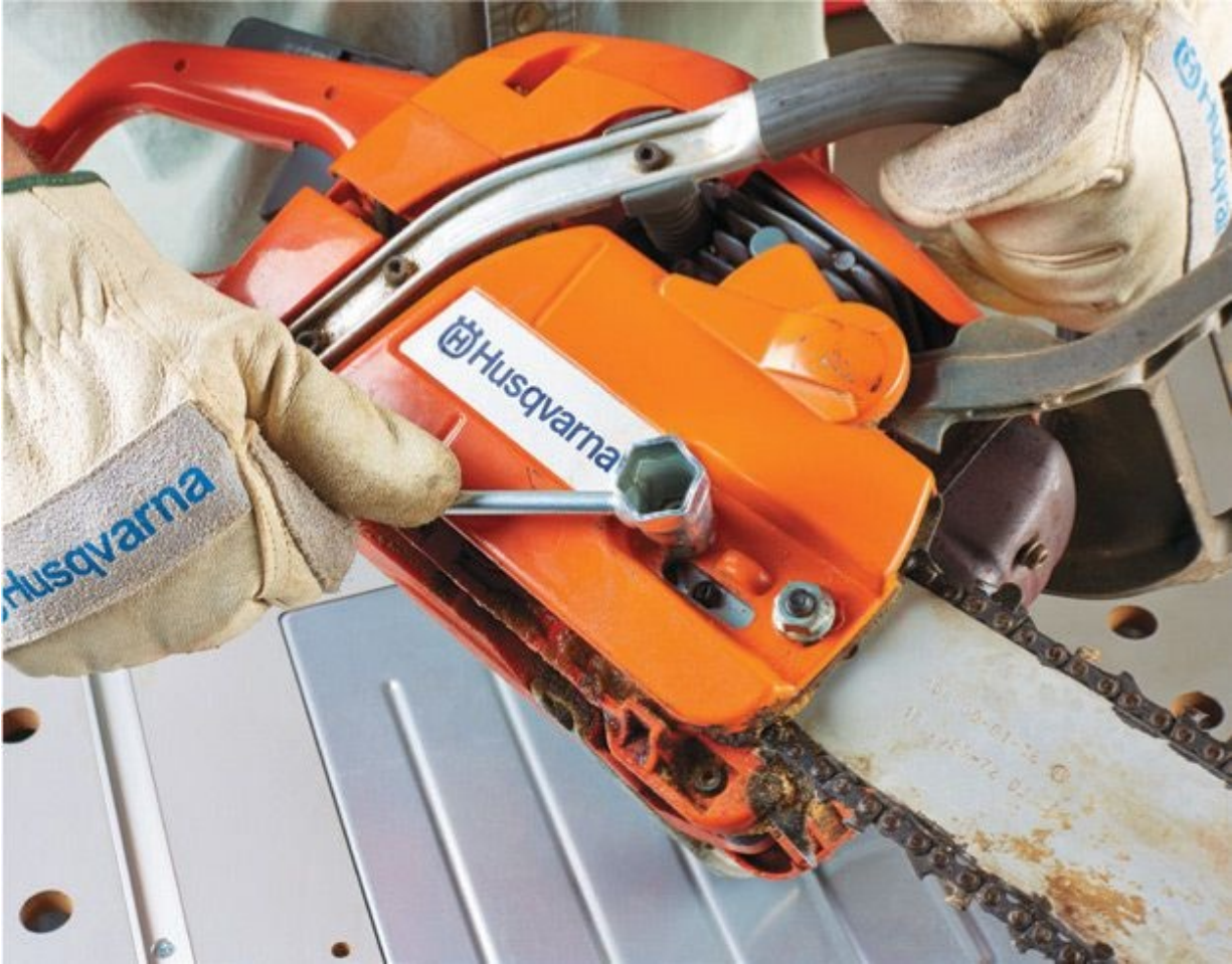
Chain tension is adjusted by loosening the bar bolts and moving the bar forward or backward.
